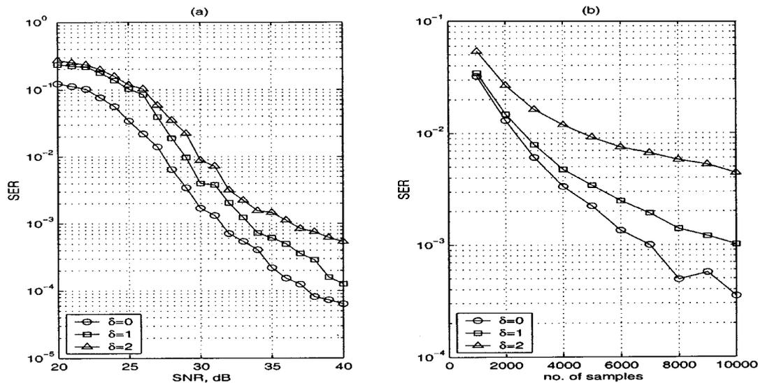
Fig. 6. Performance of the new algorithm for the nonlinear channel in Example 3. Equalizer order  $m = 2$ . (a) SER versus SNR, 5000 symbols. (b) SER versus sample size, SNR = 30 dB.
