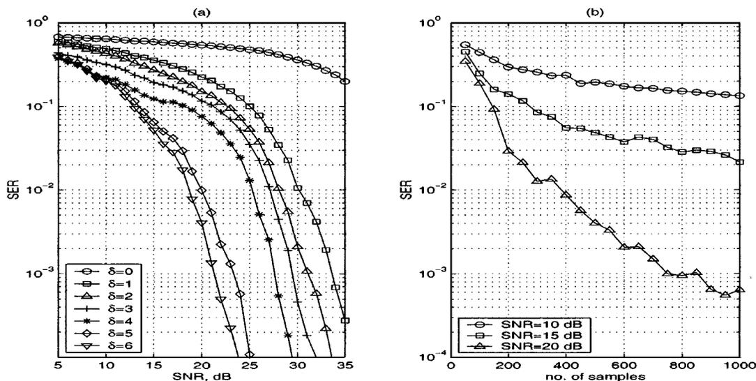
Fig. 3. Performance of the new algorithm for the nonlinear channel in Example 2, equalizer order  $m = 4$ . (a) SER versus SNR, 500 symbols. (b) SER versus sample size, equalization delay  $\delta = 6$ .
