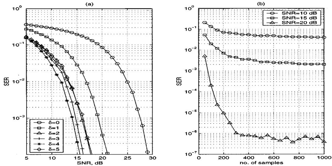
Fig. 1. Performance of the new algorithm for the nonlinear channel in Example 1, equalizer order  $m = 4$ . (a) SER versus SNR, 500 symbols. (b) SER versus sample size, equalization delay  $\delta = 5$ .
