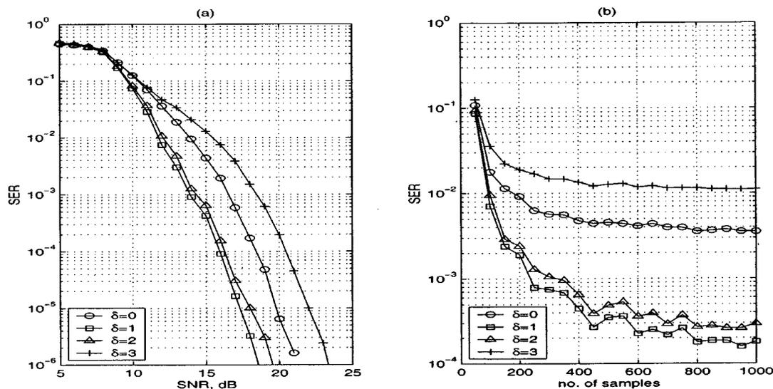
Fig. 7. Performance of the new algorithm for the nonlinear channel in Example 4, equalizer order  $m = 3$ . (a) SER versus SNR, 500 symbols. (b) SER versus sample size, SNR = 15 dB.
