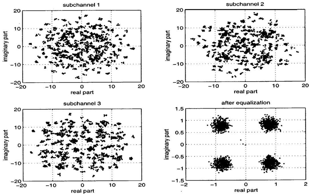
Fig. 5. Performance of the new algorithm for the nonlinear channel in Example 2: Scatter plots. Five hundred symbols, equalizer order  $m = 4$ , delay  $\delta = 6$ , SNR = 30 dB.
