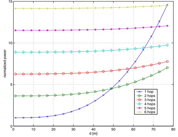
Figure 2: Power consumption for multi-hop,  $\alpha = 3$  if  $E_{RX} \neq 0$
