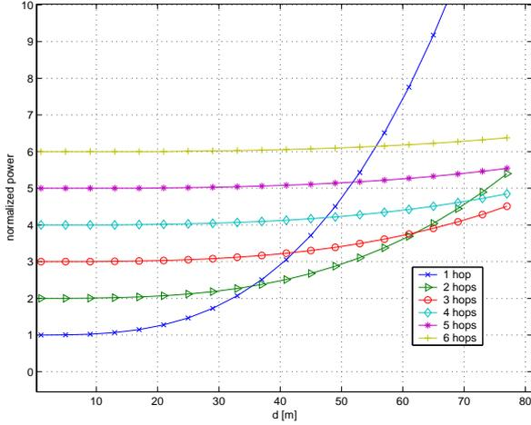
Figure 1: Power consumption for multi-hop,  $\alpha = 3$  if  $E_{RX} = 0$
