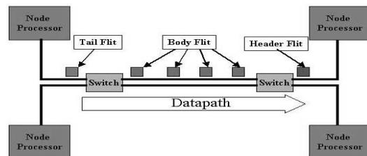
Figure 2: Flit and Wormhole Routing of Packet
