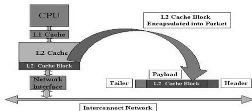
Figure 3: Packet Size and Cache Block Size
