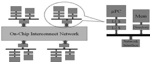
Figure 1: MPSoC Architecture
