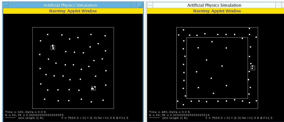
Figure 20. Simulated agents perform surveillance (left) and perimeter defense (right). For surveillance, agents are repelled by each other and by walls, while they are attracted by objects of interest. For perimeter defense agents repel each other and are drawn to the corridor between the two walls (the inner wall is porous and excess capacity is stored in the interior area). Friction is zero, because constant movement is required.
