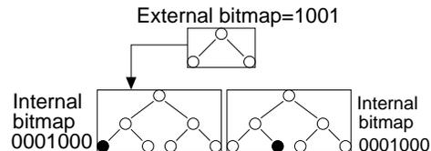
Fig. 11. This figure shows what happens if the prefixes change to 0000\* and 0010\*. Now, two child nodes are required. The external bitmap is 1001 because the first and the last child nodes of the root exist. The memory required is 73 bits.
