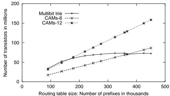
Fig. 16. The size of the routing table is increased by increasing  $C_{spawn}$ . We see that multibit tries handle this case very well.
