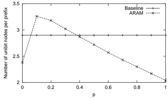
Fig. 18. This graph shows the number of unibit trie nodes per prefix as  $C_{spawn}$  is increased from 0 to 1. We see that the unibit trie density is lowest when  $C_{spawn}$  is around 0.1. This helps to calculate the worst case storage.
