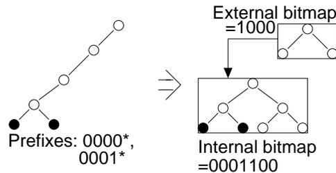
Fig. 10. This figure shows an example of a unibit trie and its corresponding multibit version for the prefixes 0000\* and 0001\*. The Eatherton bitmaps for the multibit version are also shown. The external bitmap is 1000. The memory required is 45 bits.
