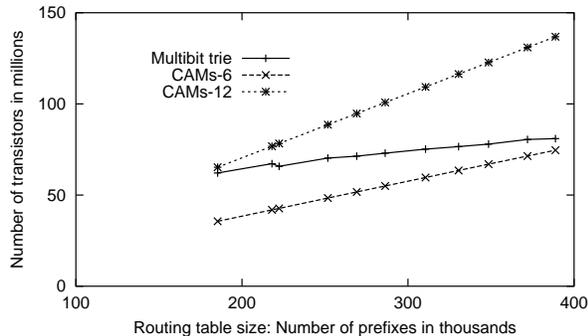
Fig. 15. The size of the routing table is increased by increasing  $F_{split}$ . We see that multibit tries scale better in this case. This is because load shared prefixes are clustered together - more than multihoming assignments.
