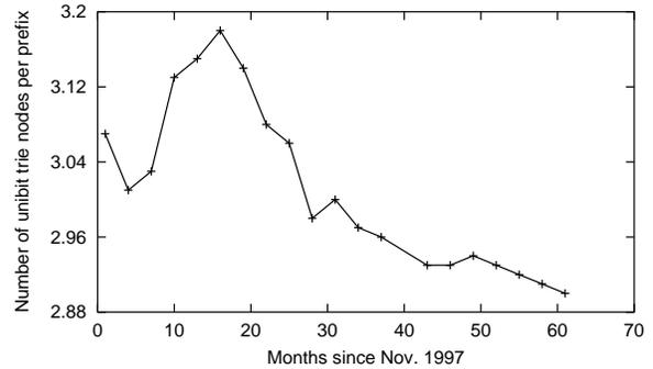
Fig. 14. The density of the trie has been increasing with time. The baseline is the number of unibit trie nodes per prefix for Nov.2002's routing table.
