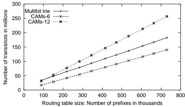
Fig. 17. The size of the routing table is increased by increasing  $F_{spawn}$ . The memory occupied by the multibit trie increases linearly with the size of the routing table.
