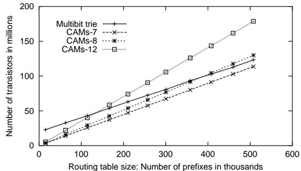
Fig. 13. The size of the routing table is increased by increasing the number of allocations. We see that unless TCAMs use 8 transistors per cell, multibit tries would eventually use lesser transistors than TCAMs.
