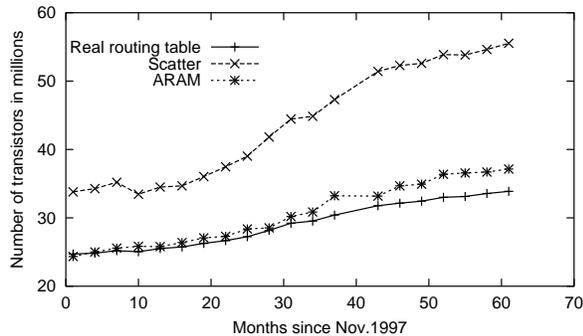
Fig. 12. The memory used by the multibit trie by the real routing table, scatter and ARAM.
