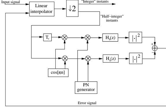
Figure 6: Block diagram of the delay-locked loop.
