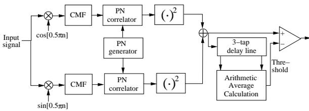
Figure 4: Block diagram of PN acquisition block.
