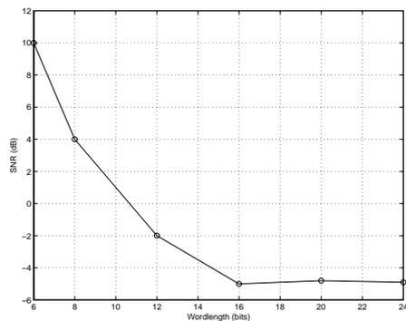
Figure 11: Simulated performance of the receiver with fixed-point operations (SNR = -5 dB).
