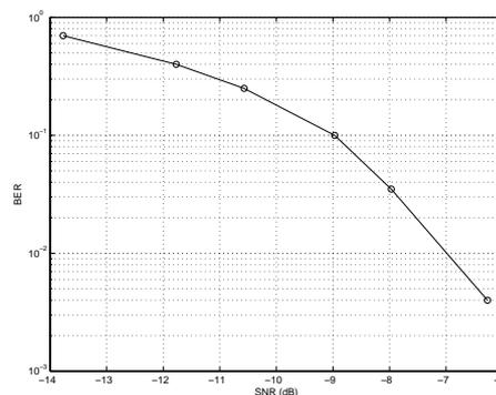
Figure 9: Simulated performance of the system with PLC noise.
