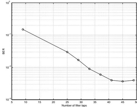
Figure 10: Simulated performance of the system versus the number of filter taps (SNR = -4 dB).
