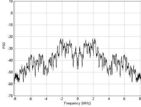
Figure 3: Example of simulated spectrum of the received signal. Note the increasing attenuation from 0 up to  $\pi$ , corresponding to the channel attenuation from 16.384 MHz up to 24.576 MHz.
