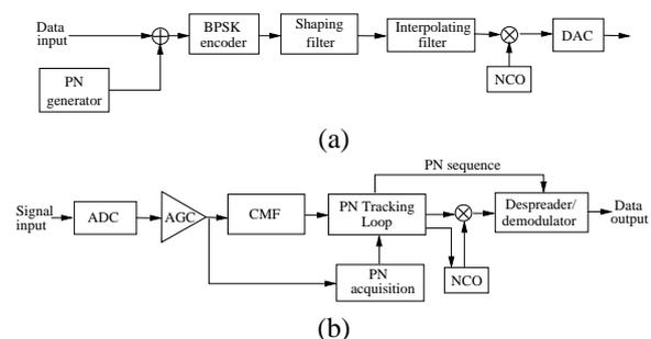
Figure 1: Block diagram of the DSSS system. (a) Transmitter block diagram. (b) Receiver block diagram.
