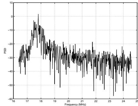
Figure 8: PLC noise PSD used in the simulations.
