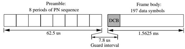
Figure 2: Frame structure. DCB denotes the DLL Convergence Bits.
