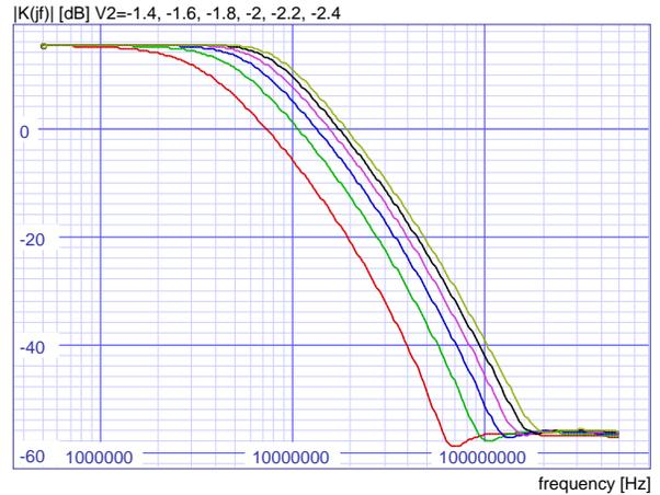
Fig. 9. Frequency responses of the new filter
