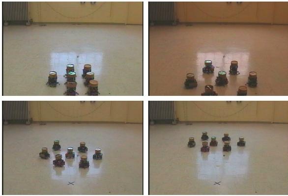
Fig. 5. Seven robots get into formation, and move toward the light.
