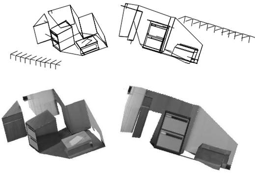
**Figure 7. Two views of the 3D point and line structure and rendered planes obtained from the first image sequence. The reconstructed camera positions are also shown.**
