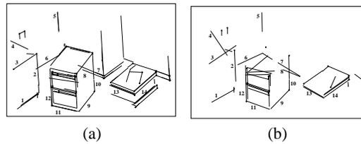
**Figure 6. 3D lines used for the evaluation of structure from motion algorithm. (a) 3D lines reconstructed with the plane constraint; (b) 3D lines reconstructed without the plane constraint.**
