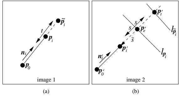
Figure 3. Epipolar constraint on junction end-points
