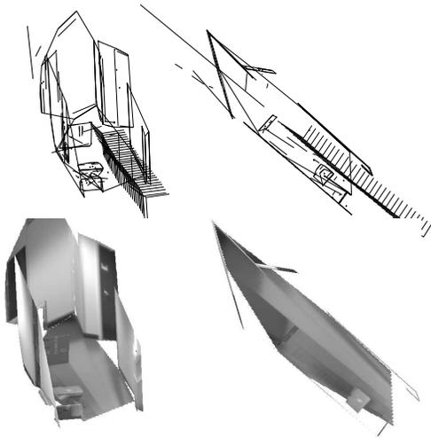
**Figure 8. Two views of the 3D structure and planes obtained from the corridor image sequence**
