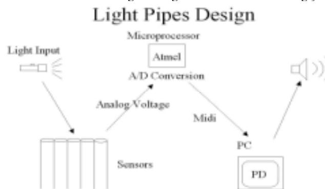
Figure 2. Light Pipes Signal Flow
