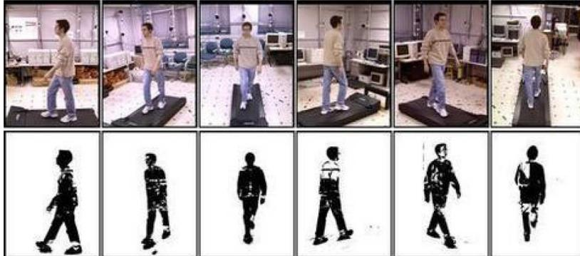
Figure 13: From [48], examples of human silhouette images (bottom) extracted using background subtraction.
