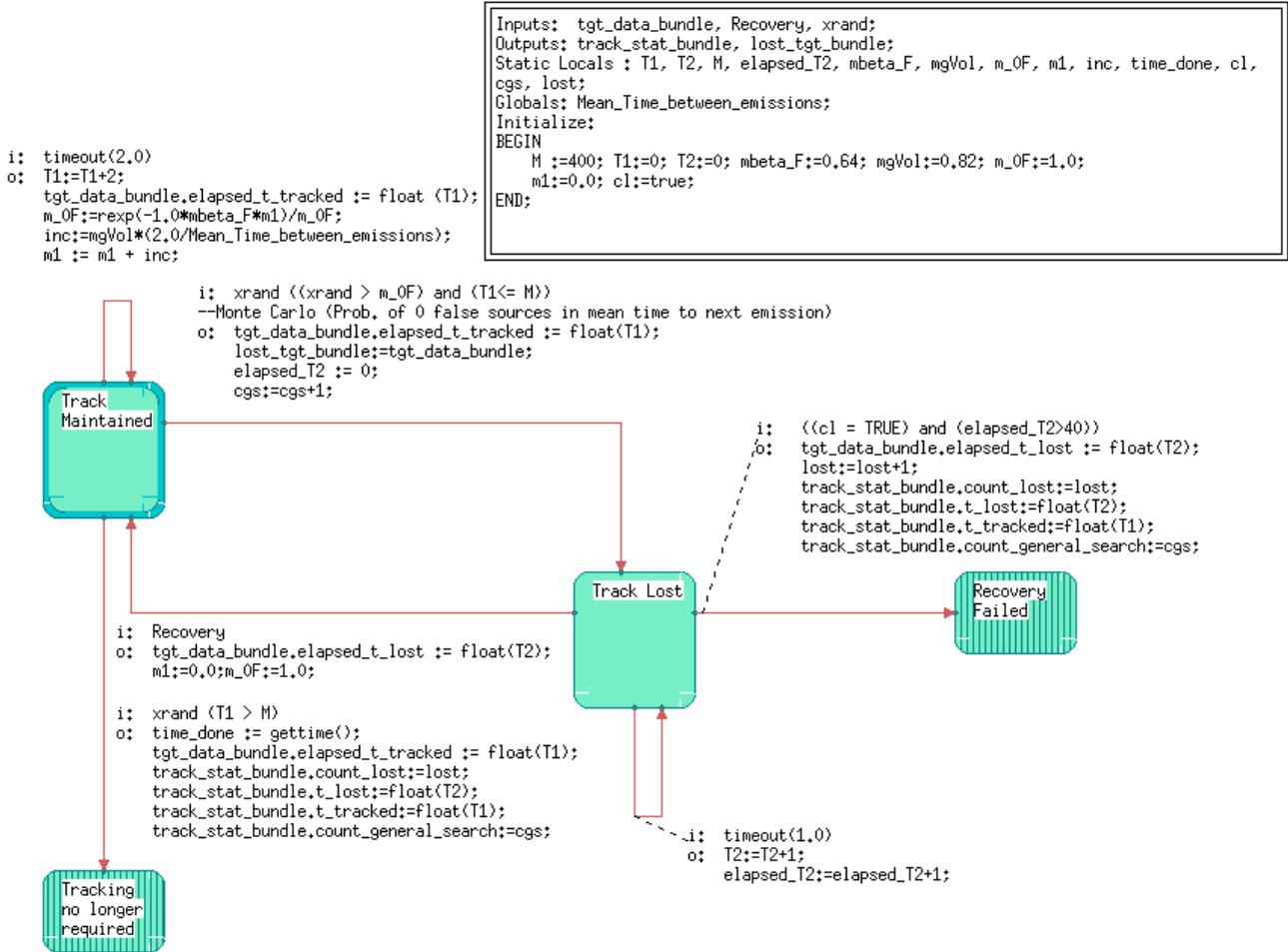
Figure 2: Track Maintenance Module
