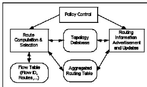
**Fig. 1.** An inter-domain QoS routing model
