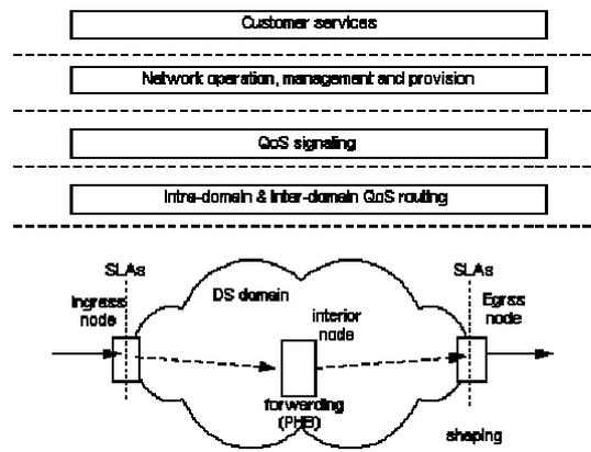
Fig. 2. DiffServ architecture with inter-domain QoS routing
