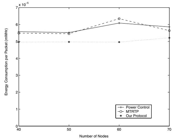
Fig. 9. Energy consumption per packet in MACA.
