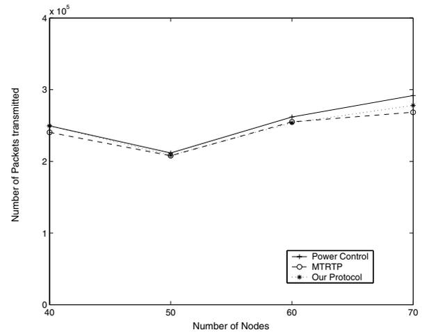
Fig. 10. Number of packets transmitted in MACA.
