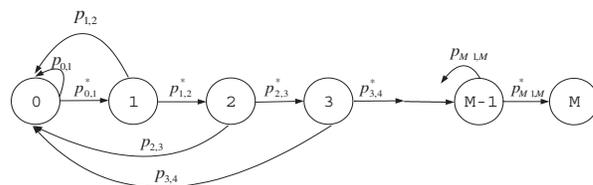
Fig. 1. State diagram for CSMA.
