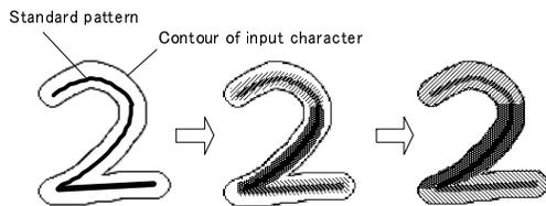
**Figure 9. Dilation of the deformed standard pattern**
