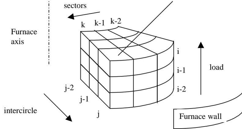
**Fig. 1 Division of blast furnace load**
