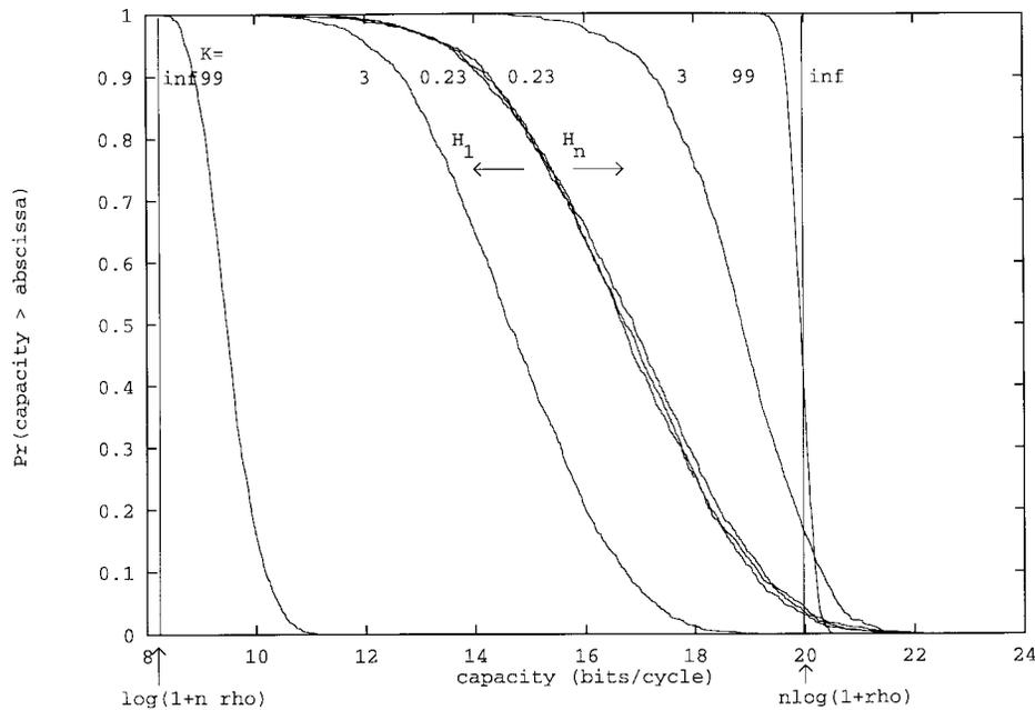
Fig. 3. Capacity on Ricean channels,  $n = 3$ .
