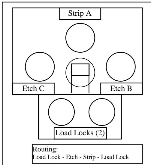
Figure 1: Schematic of a Cluster Tool
