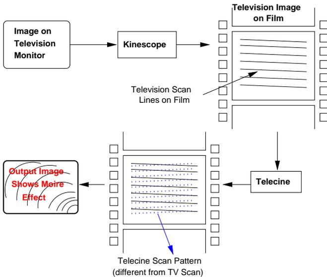
Figure 1: A block diagram of the system causing moiré degradation.
