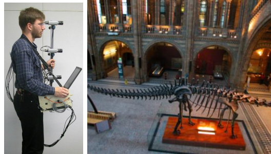
Figure 6: Left: portable multi camera image capture system, Right: Overview of the dinosaur scene being reconstructed.
