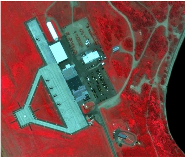
Fig. 4 – Pan-sharpened Ikonos scene subset. Near infrared, red and green displayed in RBG. 592 x 501 pixels.
