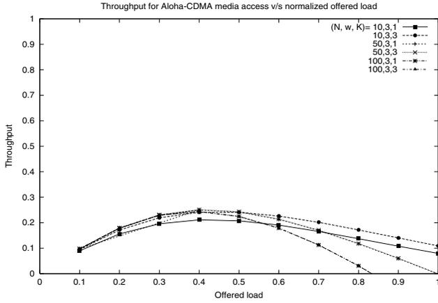
Fig. 3. Network throughput ( $T_{halo-cdma}$ ) against offered load for different codeset design parameters ( $N, w, \kappa$ ) for Aloha-CDMA from analysis. The average packet length was 500 bytes and the chipping rate was 1Gb/s.
