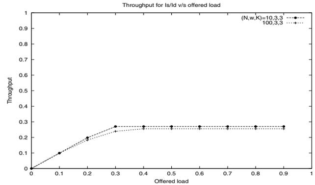
Fig. 4. Throughput for the *Is/Id* mechanism ( $Th_{isid}$ ) against offered load. The average packet length was 500 bytes and the chipping rate was 1Gb/s. The thresholds used were  $thresh_m = 2$  for both codesets and  $thresh_c=4$  for the (10, 3, 3) codeset and  $thresh_c = 40$  for the (100, 3, 3) codeset
