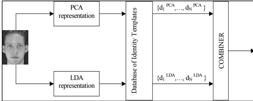
Figure #-1. The flow diagram of our Face Recognition System
