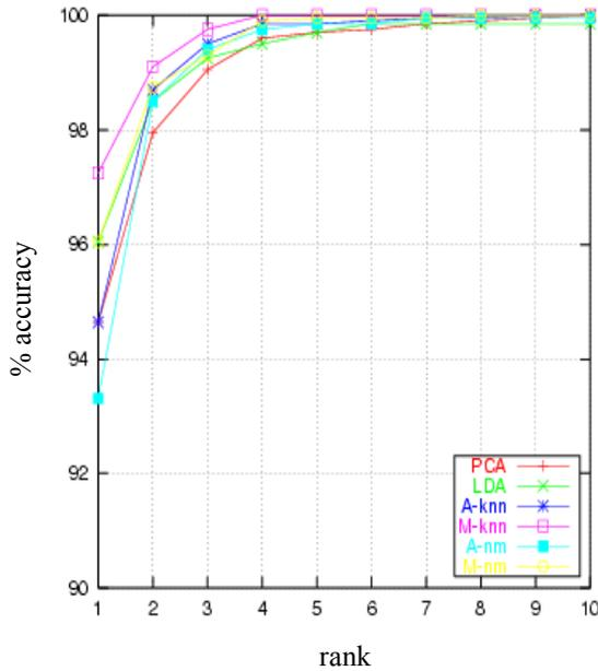
Figure #-4. Rank curves on the AT&T data set. Reported results show that the combination of PCA and LDA improves the reliability of the system
