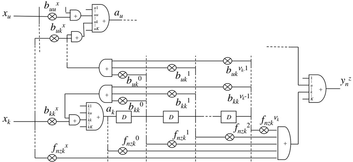
Fig. 5. The  $k$ th shift register in the constituent code.
