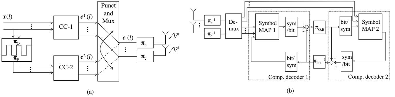
Fig. 1. System model. (a) Parallel concatenated encoder. (b) Iterative decoder.
