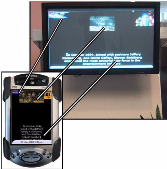
**Figure 4. The Thumbnail Model of Navigating Content.** A thumbnail version of content is displayed on the personal device enabling it to browse and exchange the content independently from the CEA.
