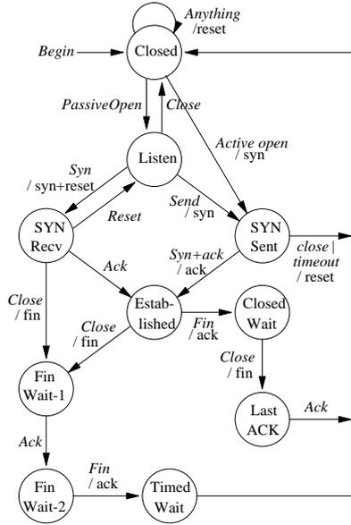
Fig. 2: State diagram of the TCP layer.
