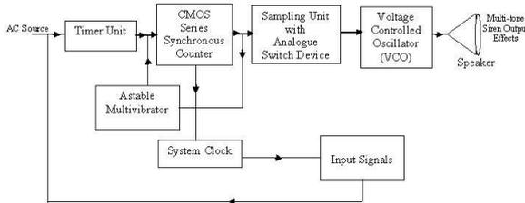
Figure 3: Simplified Block Diagram for Multi-tone Electronic Security Siren
