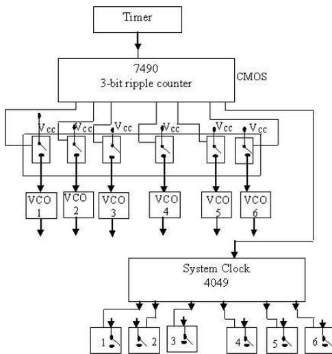
Figure 5: System clocking of the multitone siren
