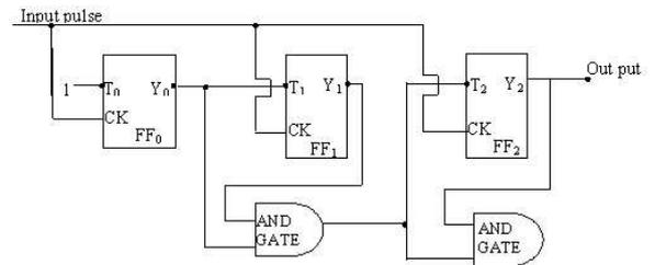
Figure 4: Series-carry synchronous counter for 3 bit ripple counter.
