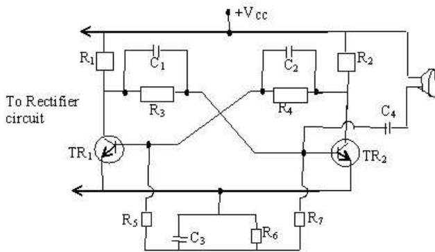
Figure 1: Astable multi-vibrator producing multitone siren effect.
