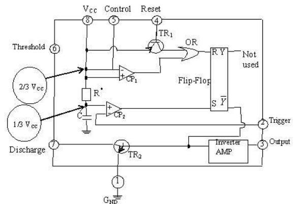
Figure 2: 555 Timer Configured into astable multi-vibrator.
