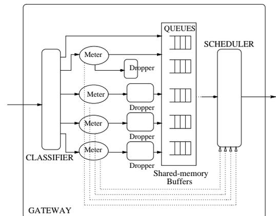
Fig. 7. The Structure of the DiffServ-based Backbone Router.
