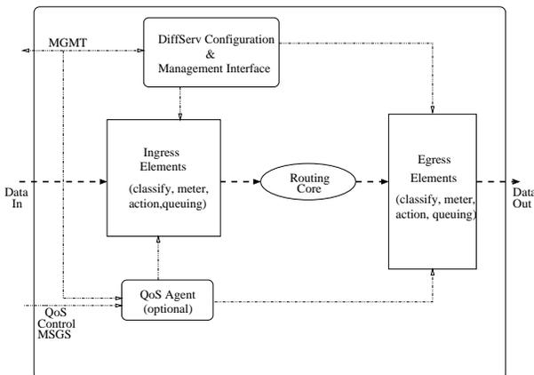
Fig. 4. High Level View of a DiffServ Router.
