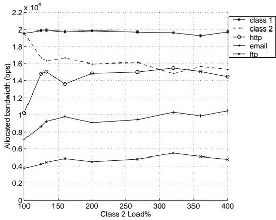
Fig. 9. Allocated bandwidth allocated vs. G2 load%.
