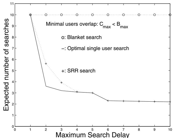
Fig. 1. The expected number of searches per user, as a function of the maximum search delay deadline, for small users location overlap.
