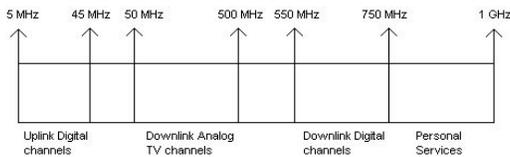
Fig. 3.1 Frequency Spectrum of HFC [13]
