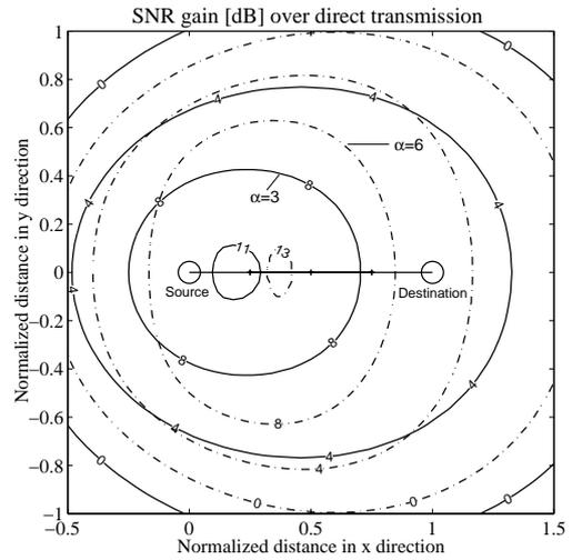
Figure 6: Usage region of the detached cooperative diversity protocol for  $R=2$  bit/s/Hz, frame error rate  $p^{out} = 10^{-2}$ ,  $N = 100$  and  $\alpha = 3$  (solid lines) as well as  $\alpha = 6$  (dash-dotted lines). It is clearly more favorable to place the relay close to the source, for low values of  $\alpha$ .
