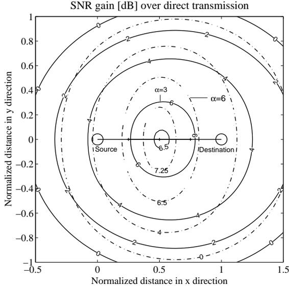
Figure 4: Usage region of the detached cooperative diversity protocol for  $R=2$  bit/s/Hz, outage probability  $p^{out} = 10^{-2}$  and  $\alpha = 3$  (solid lines, rural environment) as well as  $\alpha = 6$  (dash-dotted lines, indoor environment). The radius of the usage region lies in the order of the source-destination distance.
