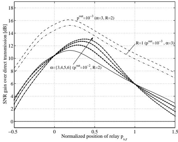
Figure 5: SNR gain of the detached adaptive decode-and-forward protocol over direct transmission for  $N = 100$ . The maximum SNR gain as well as the optimal relay position depend significantly on  $\alpha$ . For low values of  $\alpha$ , the relay should be close to the source while for high  $\alpha$  it should be placed halfway between source and destination. Spectral efficiency and required FER have no influence on the spatial distribution of the SNR gain.
