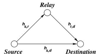
Figure 1: Illustration of a cooperative diversity scenario. The source sends a broadcast message to destination and relay. The relay then forwards an additional copy of the source message to the destination, which appropriately combines the two messages.
