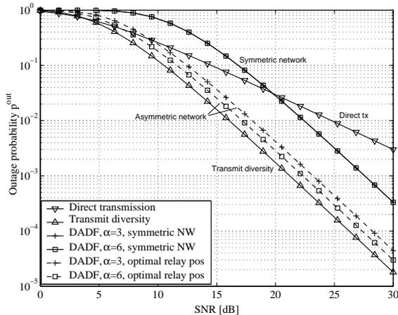
Figure 2: Performance of the detached adaptive decode-and-forward protocol in terms of outage probability versus SNR for spectral efficiency  $R=2$  bit/s/Hz. Full second order diversity is achieved in all network constellations. The most substantial gains over direct transmission can be obtained by placing the relay halfway between source and destination (i.e.,  $r_{s,r} = r_{r,d} = 0.5$ ).
