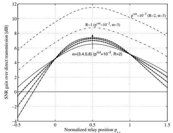
Figure 3: SNR gain of the detached adaptive decode-and-forward protocol over direct transmission.  $r_{s,r}$  denotes the position of the relay between source and destination, normalized to the source-destination. The maximum SNR gain is obtained for  $r_{s,r} \approx 0.5$ , independent from  $\alpha$ . Spectral efficiency and required outage probability have no influence on the spatial distribution of the SNR gain, which is only influenced by  $\alpha$ .
