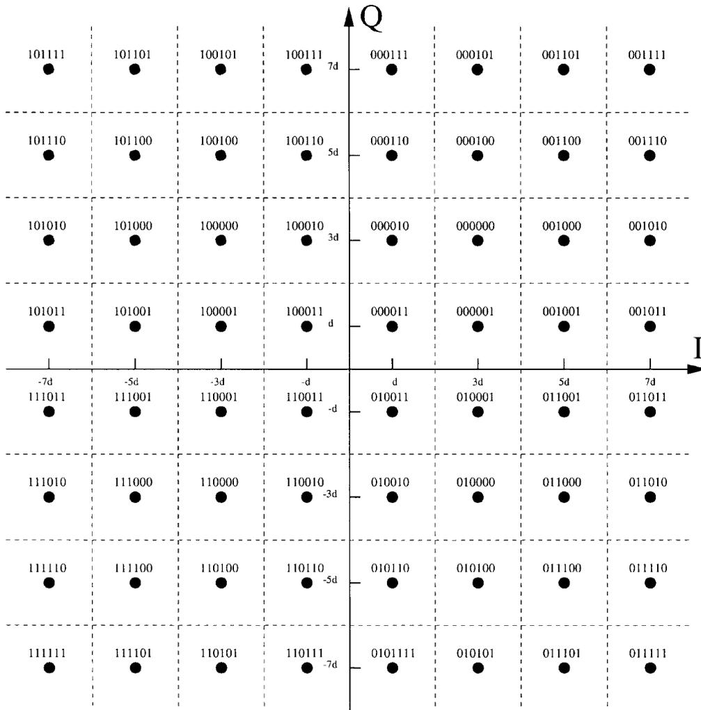
Fig. 4. 64-QAM constellation with Gray encoding.
