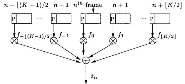
Fig. 8. Fading interpolation in PSAM.
