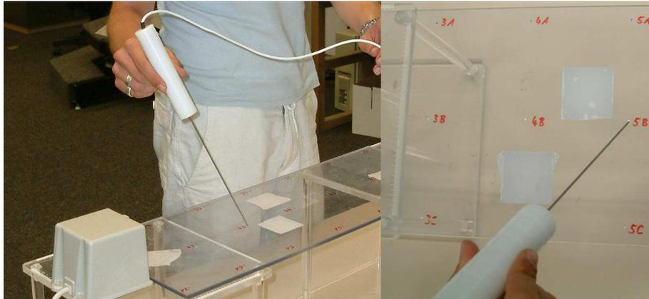
**Figure 5.** Measurements are recorded with instrument tip at one fixed point and sensor embedded in the instrument handle that is being moved around.
