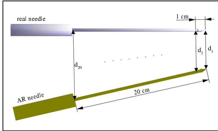
**Figure 9.** The distances between equally spaced positions at the axes of real and AR needle have been calculated. Samples on twenty such positions spaced at 1 cm have been taken – beginning at the needle’s tip ( $d_1$ ) and moving 20 cm up towards the handle.
