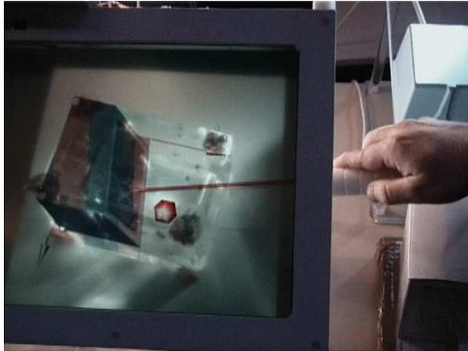
**Figure 1.** The transparent AR display developed for the MEDARPA system. A rendered scene based on CT data of a phantom can be seen. The phantom itself can be perceived through the display.
