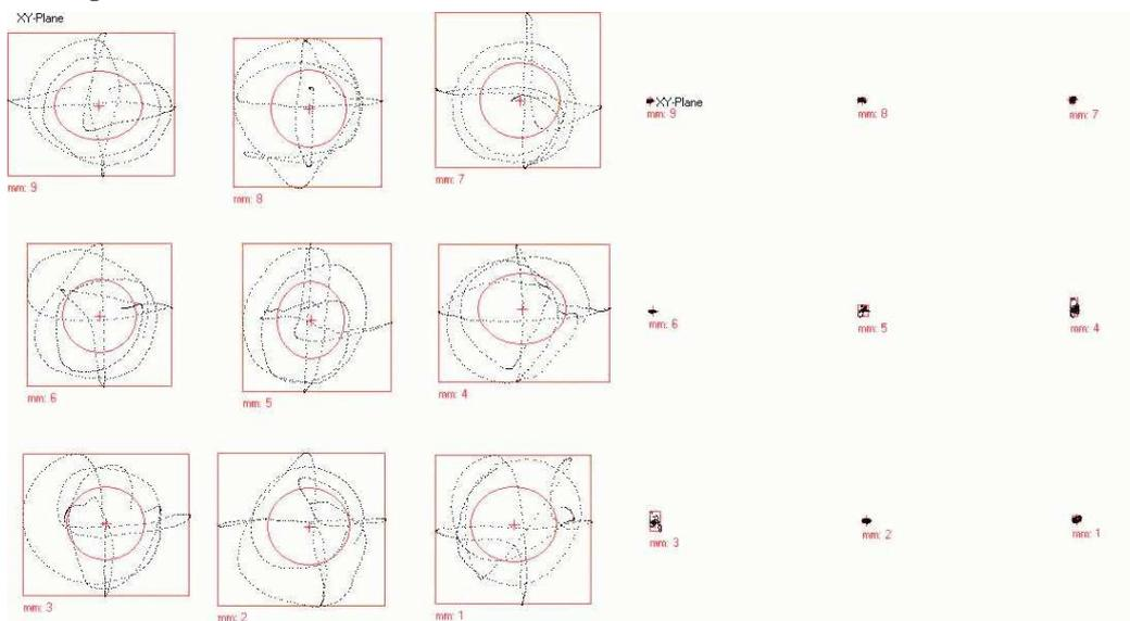
**Figure 6.** Recorded measurements with the instrument's tip at one fixed point and the sensor embedded in the instrument handle moved around. The positions projected onto the XY-plane are displayed. On the left side the raw measurements delivered by the electromagnetic tracking are shown, on the right side the same measurements after applying the calculated offset transformation are presented.
