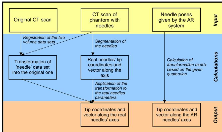
**Figure 8.** Data flow of the calculation process: the input data is used for the calculation of the real and AR needles' poses in the frame of reference given by the original data set.
