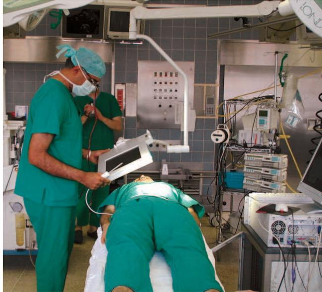
**Figure 2.** Setup of the MEDARPA system for evaluation in an operation theatre.
