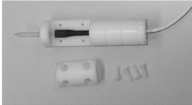
**Figure 3.** Instrument for registration with integrated sensor. The offset between the tip and the sensor has to be determined. A similar handle with an integrated sensor is used for embedding the brachytherapy needle.
