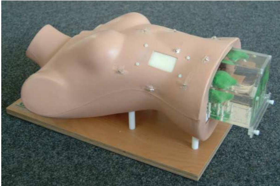
**Figure 7.** The anthropomorphic phantom. It contains a cuboid-shaped acrylic form similar to those used for the accuracy tests.
