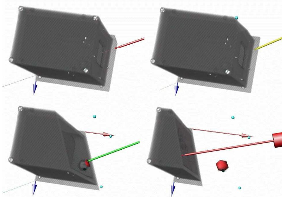
**Figure 4.** Four steps of navigation(left to right, up, down): searching for target direction, going along direction to target, collision with target, undetermined state.
