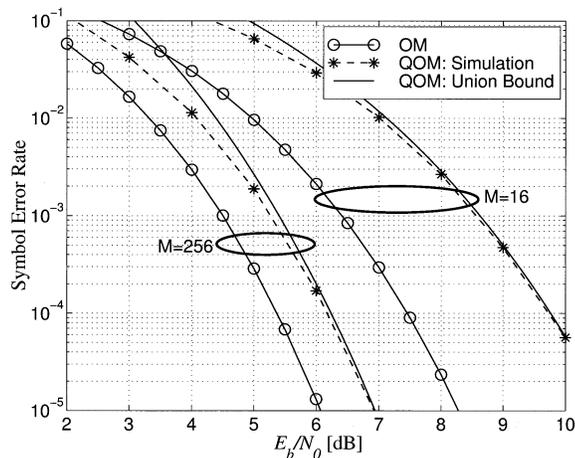
Fig. 1. SER performance of OM and QOM under AWGN with noncoherent demodulation.
