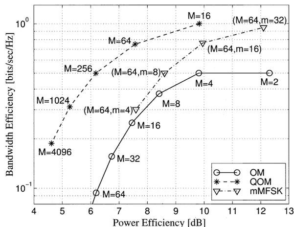
Fig. 2. Bandwidth efficiency vs. power efficiency under AWGN.
