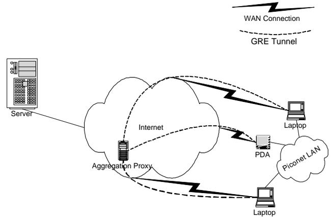
Fig. 1. A bandwidth aggregation service architecture.
