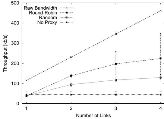
Fig. 10. Effect of piconet size on TCP throughput.
