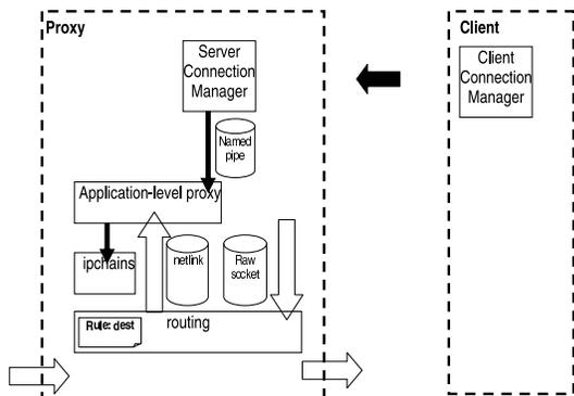
Fig. 8. Linux-based implementation of an aggregation proxy.
