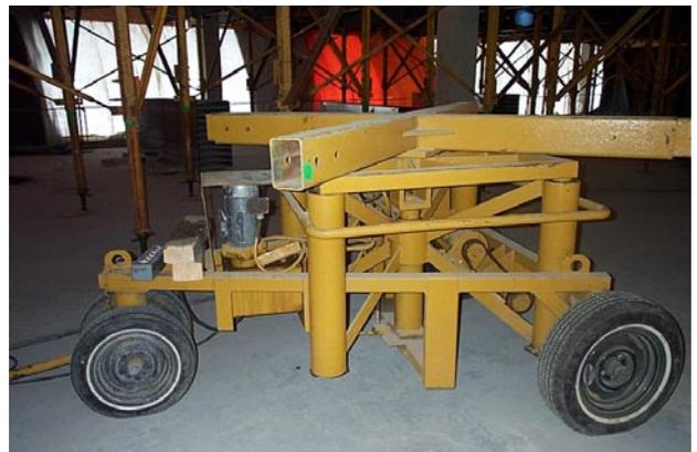
Figure 4: Portable Jack Used for Slab Fly Form Transport
