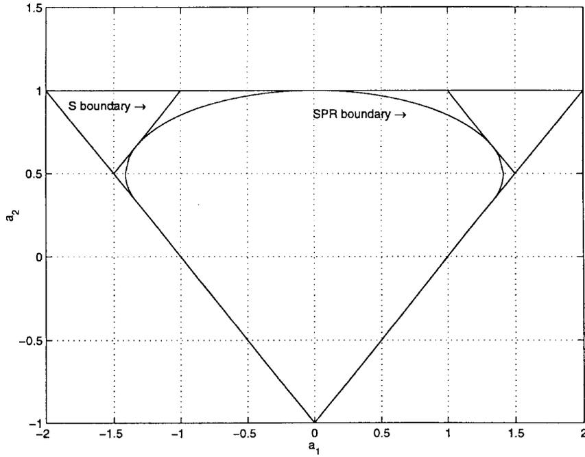
Fig. 2. The set  $\mathcal{S}$  for  $n = 2$ . Also displayed are the stability triangle and the SPR region.
