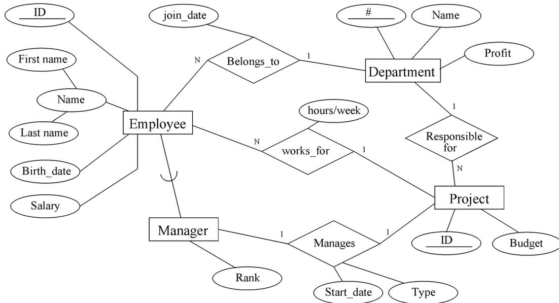
Fig. 10. A TEER schema modeling the running example.
