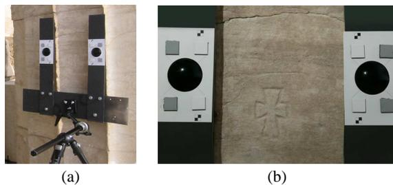
Figure 1: (a) The adjustable light-capturing frame includes fiducial markers, reflectance standards and two glossy black spheres. (b) One of the input image for an inscription on a column of the Parthenon.
