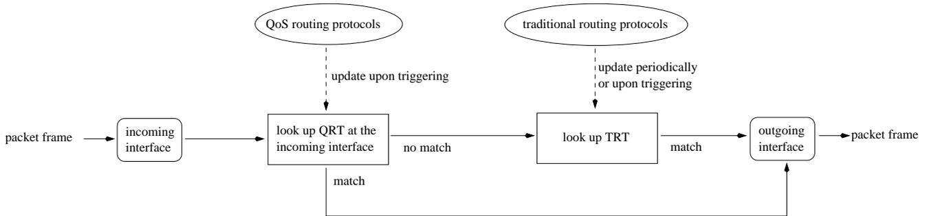
Figure 1. TRT and QRT: When an EF packet arrives, the QRT at the incoming interface is first looked up. If there is a match, the packet is forwarded to the next hop and the TRT is not checked; otherwise, the TRT is looked up.
