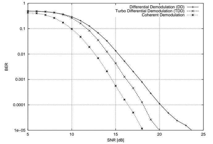
Fig. 5. BER for 16-DAPSK in an OFDM transmission scheme (No. of Subcarriers: 1024, Coh. Bandwidth: 190 kHz, Subcarrier Spacing: 4 Khz, Bit Interleaver Length: 4048, NLOS)
