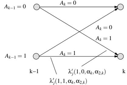
Fig. 3. Amplitude Trellis for TDD of 16-DAPSK
