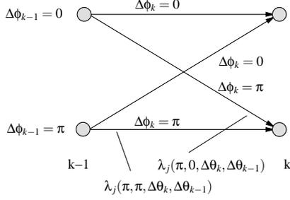
Fig. 1. Trellis diagram for MSDD of binary DPSK
