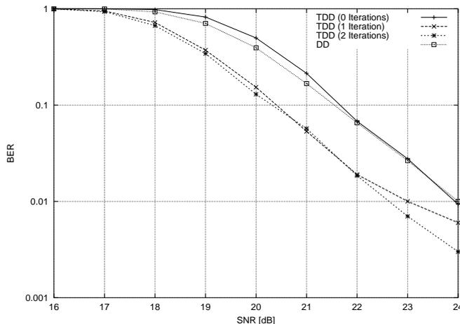
Fig. 7. PER for 64-DAPSK in an OFDM transmission scheme (No. of Subcarriers: 2048, Coh. Bandwidth: 190 kHz, Subcarrier Spacing: 4 KHz, Bit Interleaver Length: 12282, LOS (8 dB))
