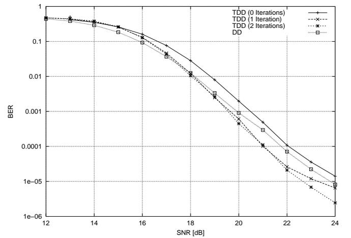
Fig. 6. BER for 64-DAPSK in an OFDM transmission scheme (No. of Subcarriers: 2048, Coh. Bandwidth: 190 kHz, Subcarrier Spacing: 4 Khz, Bit Interleaver Length: 12282, LOS (8 dB))
