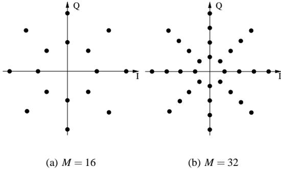
Fig. 2. Signal space diagram for DAPSK
