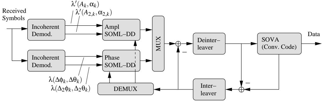
Fig. 4. Block diagram of iterative detection algorithm
