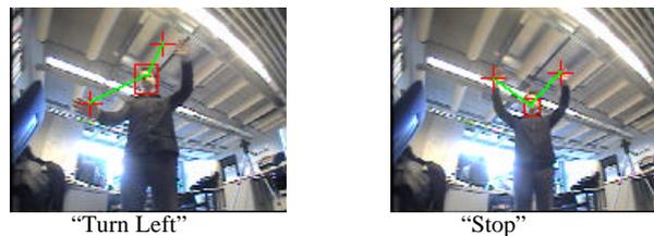
Fig. 7. Static gesture recognition for robot motion control
