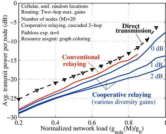
Fig. 3. Average transmit power per node as a function of the normalised network load. Cellular scenario with 20 users per cell.
