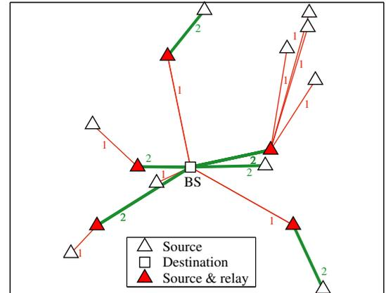
Fig. 2. Example of a cellular network with 15 nodes and a central base station. Two-hop max gains routing. Resources (time slots or frequencies) are indicated with different line colors, thicknesses and labels.
