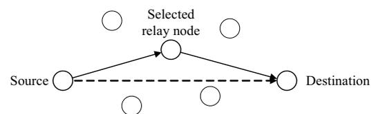
Fig. 1. A possible two-hop relaying scenario. Conventional relaying occurs along the solid arrows. In cooperative relaying, the destination additionally takes the signal sent by the source into account (dashed-line arrow).
