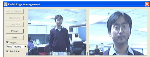
Fig 4. An example of attention based video adaptation. The human faces are detected in the video stream and only those regions are delivered to the client device. Therefore, he/she can see a more clear face image on the small screen and the bandwidth cost can also be reduced.
