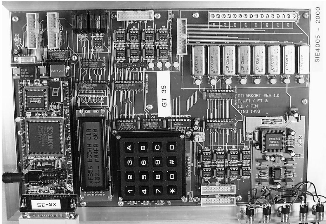
**Figure 4.** A picture of the lab board developed for use in the course *SIE4005 digital design and computer fundamentals* at NTNU.
