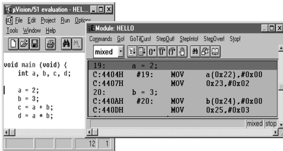
**Figure 3.** User interface of the Keil C compiler showing C code compiled to assembly code running on the 8051 microcontroller.
