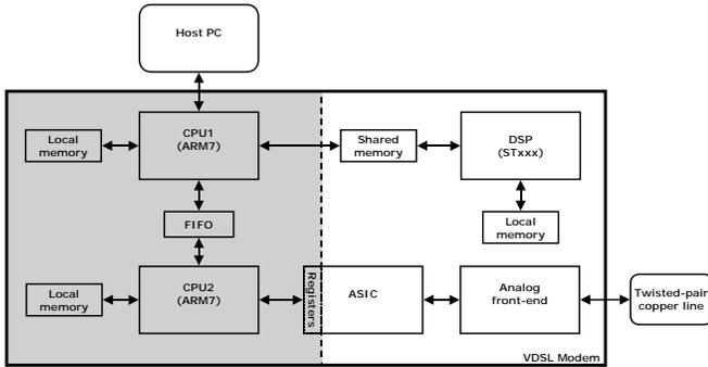
Figure 9: VDSL modem application.
