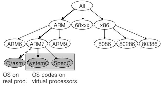
Figure 4: An example of processor dependency.
