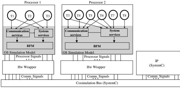
Figure 2: Timed cosimulation models of VDSL modem application.
