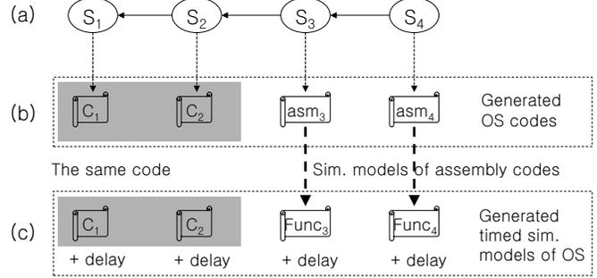
Figure 5: Examples of OS codes and simulation models.
