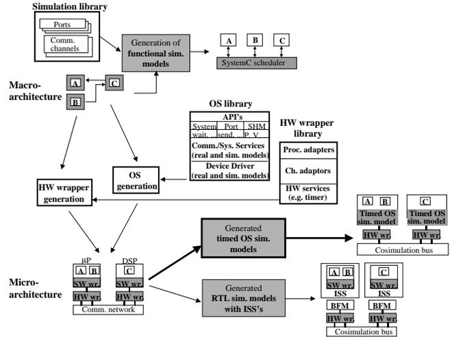
Figure 1: Micro-architecture generation flow.
