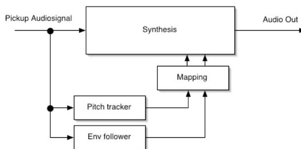
Figure 1: basic principle of the algorithm
