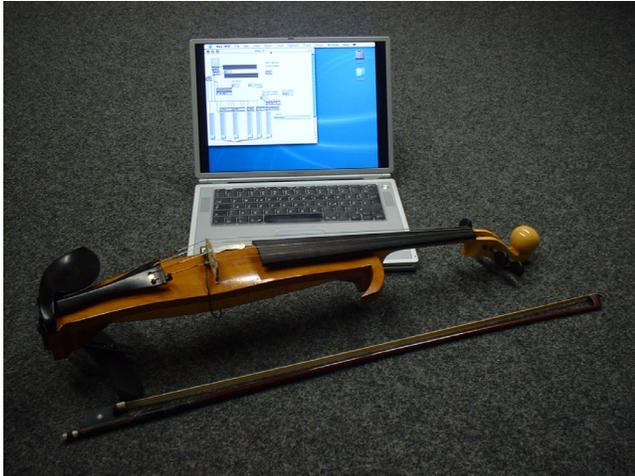
Figure 2: Example of the complete hardware needed: Mac PB G4 and Harms silent viola with pickup
