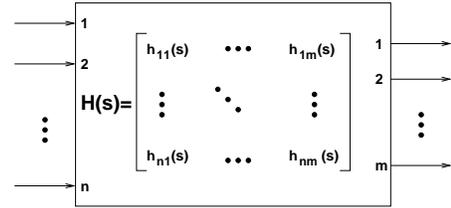
Figure 5: Transfer function of an interconnect network
