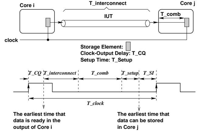
Figure 14: The effect of interconnect skew (delay).
