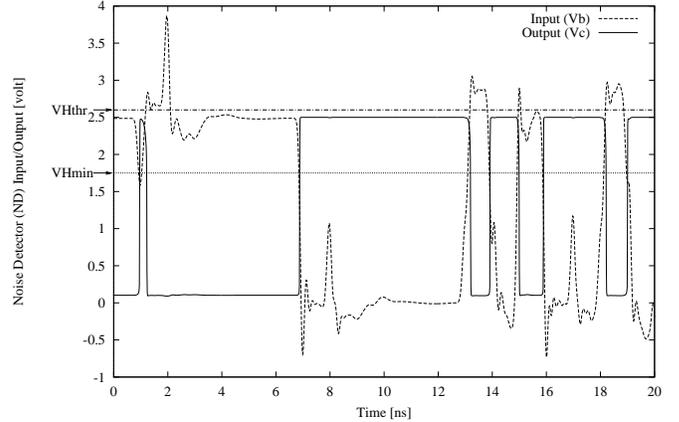
Figure 11: The SPICE simulation of the ND cell for the top vulnerable region.
