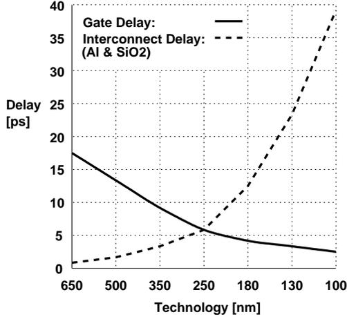
Figure 13: Gate and interconnect delay versus technology.
