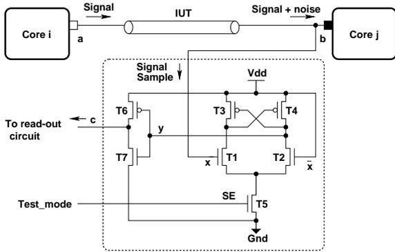
Figure 10: The ND cell using cross-coupled PMOS amplifier.
