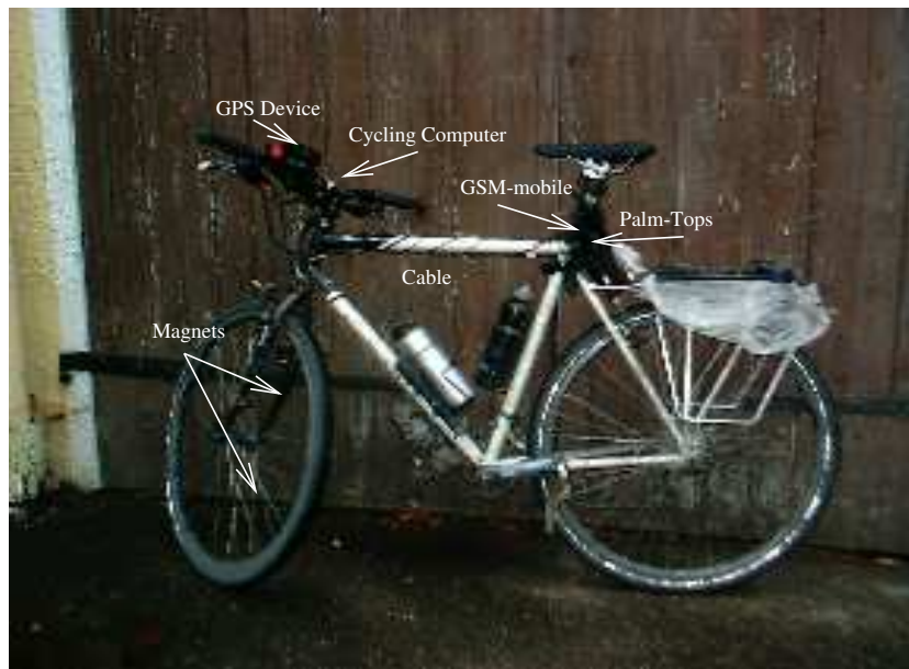
Fig. 2. A bike equipped to gather GPS data.
