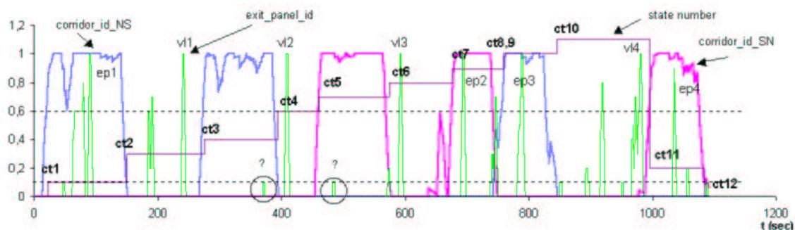
Figure 5: Landmark identification state of a complete path that amounts to 149.5 meters. The circles show the missed exit pannels in that corridor. The stairs-like line displays changes in the state number (multiplied by 0.1 for scale purposes). These changes show that the complete state sequence that corresponds to the defined full path, has been met. The state numbers are those drawn in the FSA.
