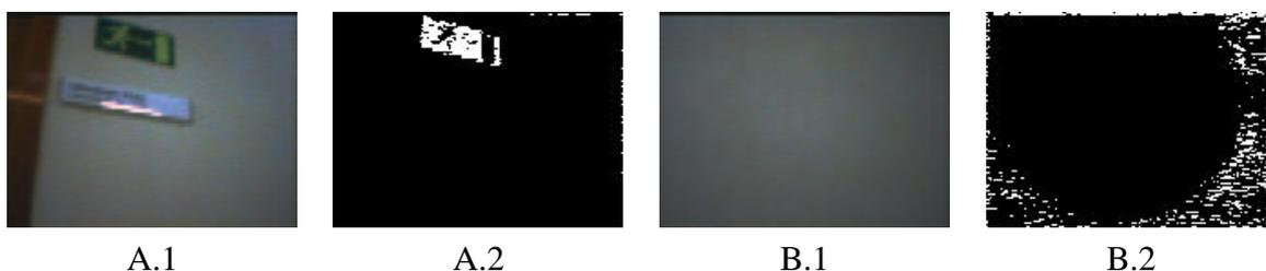
Figure 2: Original and segmented images. The green emergency panel on image A.1 gives a good segmented result as shown in image A.2. Image B.1 is an original image with no panel and B.2 shows the noisy segmented image obtained.
