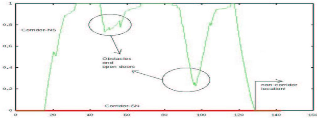
Figure 3: Capture of the corridor identification state during a NS corridor. The thick line around 0 value represents the identification state of the SN corridor. Circles underline perturbances.
